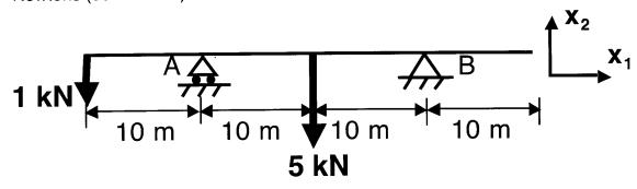
(a) Determine the reaction forces at support points A and B *or* indicate all information available to determine the reaction forces and the additional information that is needed to fully determine these forces.
