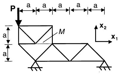
(a) What is the "class/category" of this structural configuration (Dynamic, Statically Determinate, Statically Indeterminate)? Clearly explain your reasoning.
