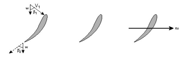
a) Draw velocity triangles in the relative and absolute frames for the different blade speeds shown below for both the inlet and exit to the rotor. (Note the inlet velocity components form a 3-4-5 triangle.)
