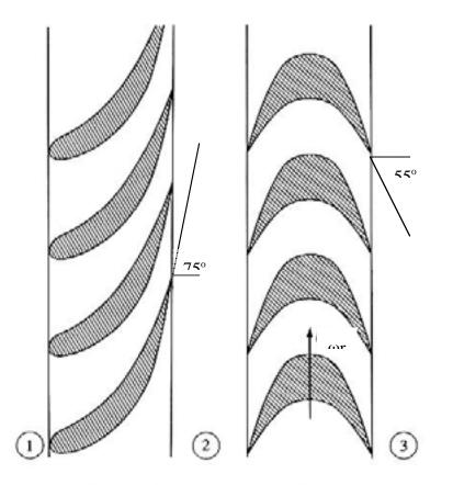
a) Neatly draw and label the velocity triangles assuming the blade speed  $\omega r = 2w$ , where w =100 m/s is the axial velocity.
