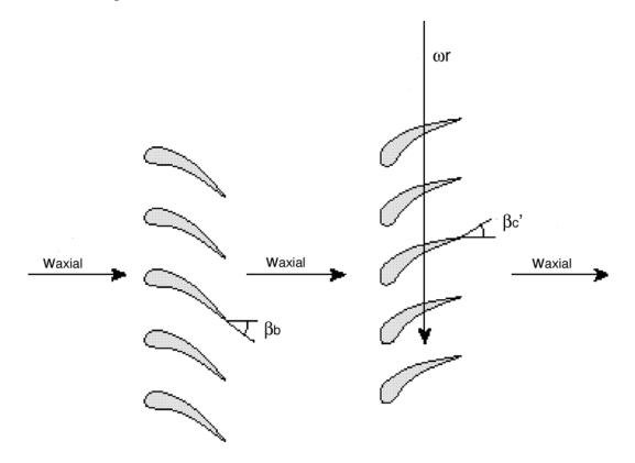
b) Say in words what the torque is equal to. Write an expression for the torque on the first blade row and draw the direction of the force experienced by the blades in the first row.
