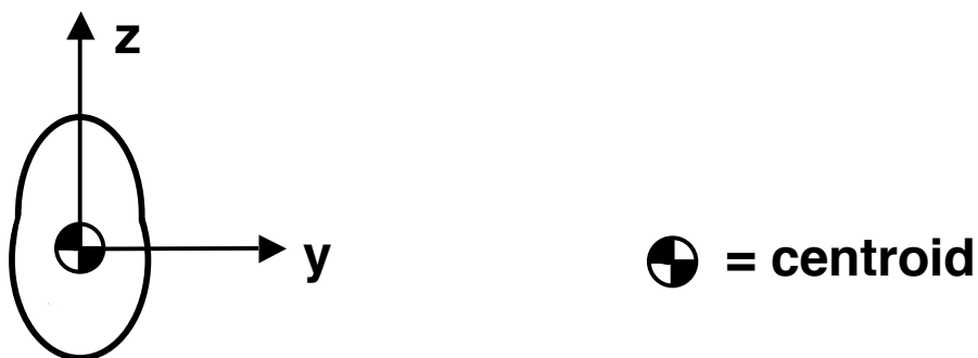
Figure M4.5-3 General cross-section with axes recounted at centroid
