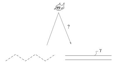
3) Now determine and sketch the velocity field of the two vortex sheets. Explain how this velocity field, which is set up by the tail, is consistent with the tail acting as a propulsor. Hint: If it helps, qualitatively compare the velocity field of the sheets to the velocity field behind a jet engine.
