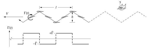
We now wish to examine the velocity field of the vortices left behind by the dolphin. To do this, we will "smear" the discrete vortices into two continuous vortex sheets parallel to the dolphin's path, with constant strengths  $\gamma = +\gamma_s$  and  $\gamma = -\gamma_s$ .
