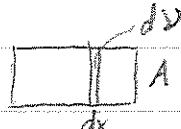
$$E_{kin} = \int_{-L/2}^{L/2} \frac{1}{2} \rho \left( V_{avg} - \Delta V \frac{x}{L} \right)^2 A dx$$
