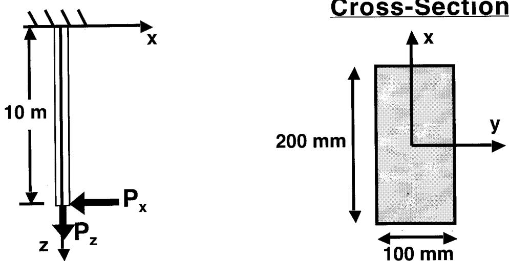
The structural configuration is subsequently *also* subjected to a vertical tip load,  $P_z$ , of 400,000 N.
