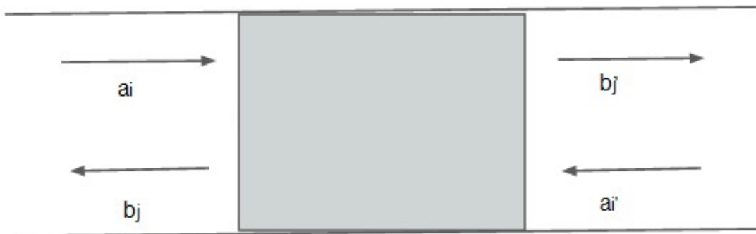
Figure 1, Scattering process. a_i is the amplitude of incoming wave from the left, b_j is the amplitude of the reflected wave from the left. Similarly, a_i^* and b_j^* have the same meaning except that they are from the right side.
