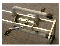
Ergonomic pump mechanism allows for steady pumping with minimal effort. Low-tolerance diaphragm pumps can take the daily abuse of farm life.
