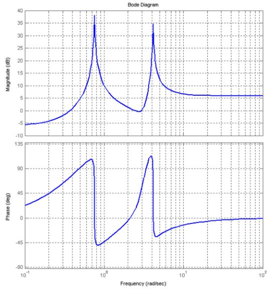
If this is used as PID controller the frequencies reduced will be those of the peaks of the magnitude response. Namely  $\omega=0.75$  rad/s and  $\omega=4.1$  rad/s
