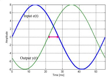
The distance shown is how much the output would need to shift to be at a phase of 180°, in other words this is our phase margin. By estimating this shift from the graph and converting it to degrees, we get that the shift margin is  $\Phi_M \cong 40^\circ$ .
