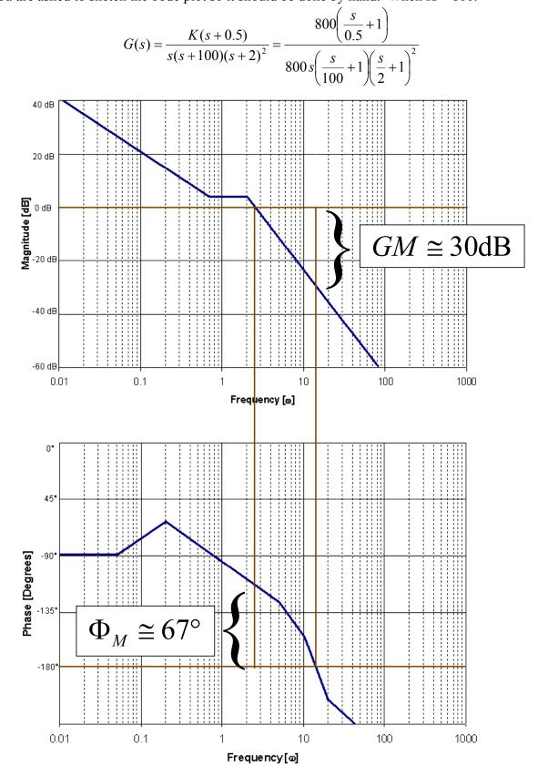
The gain margin of 30 dB implies that the entire magnitude curve can be shifted up by 30 dB, which is the equivalent of lowering the 0 dB mark by 30 dB. Since we can shift the curve by up to 30 dB that means that the gain can increase from what it is now by a factor of up to:  $20\log(\text{gain}) = 30 \text{ dB} \implies \text{gain} = 31 \text{ times}.$
