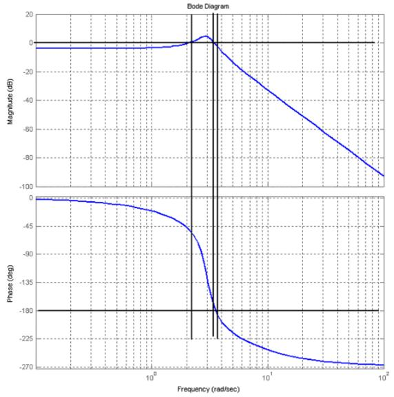
Though it is difficult to see using matlab we find that when the phase crosses  $180^{\circ}$  at  $\omega = 3.55$  rad/s the magnitude is -1.2 dB, so the phase margin is 1.2 dB.
