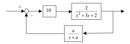
The first step here is to find the closed loop transfer function for the system, which reduces to:
