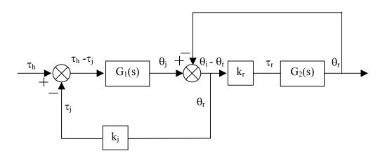
Again, the first thing we do, is to find the transfer function between  $\frac{\theta_j}{\tau_h}$ , assuming that we have not yet applied the proportional-derivative control. which we will do in exactly the same method used in part a). by first finding the  $\frac{\theta_r}{\tau_h}$  transfer function and then
