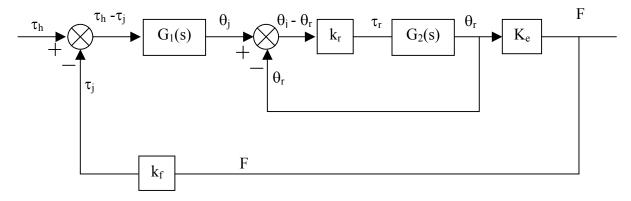
The block diagram as shown has all the connections described by the equations. For instance notice that  $\tau_j = -k_j(\theta_j - \theta_r)$ , is created around the second summing junction.  $G_1(s)$  and  $G_2(s)$  represent the characteristic of each arm. For  $G_1(s)$  we need to find the transfer function between  $\tau_h$  -  $\tau_j$  and  $\theta_j$ , while for  $G_2(s)$  we need to find the transfer function between  $\tau_r$  and  $\theta_r$ .
