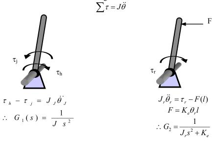
Now we can start simplifying the block diagram to get the response. The easiest way to do this is to find the transfer function  $\frac{F}{\tau_h}$  and then find the transfer function  $\frac{F}{\theta_j}$  and then
