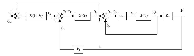
Here is the new block diagram including the proportional-derivative control. Now we are looking for the transfer function:  $\frac{\theta_j}{\theta_h}$ . Again, we could reduce the block diagram to find
