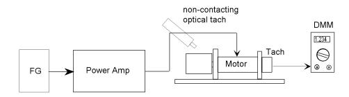
**Procedure:** With the setup as before, remove the torque monitoring lever arm and connect your DMM to the tachometer BNC connector on the motor terminal box. Apply a small dc voltage using the function generator and let the motor spin. The lab instructor will help you to measure the angular velocity with a non-contacting optical
