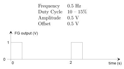
Use the square wave to drive the motor, and record the square wave on Ch. 1 of the oscilloscope, and the angular velocity  $\Omega$  from the tachometer on Ch. 2 of the scope. Adjust the duty cycle to ensure that the motor comes to rest between pulses. Which model of the friction best describes the observed velocity response? Write your answer with reasons below:
