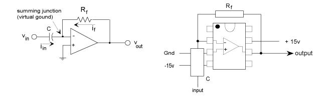
Use a 4.7  $\mu$ F capacitor and a 10K resistor. Compute the transfer function of the differentiator.
