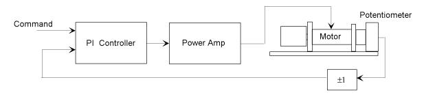
Use the function generator and the oscilloscope to record the step response of this system. Explain your observations in terms of a root-locus.
