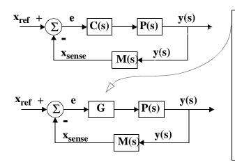
For a "proportional" feedback controller, "C(s)" is just "G" (a constant). The resulting control system simply multiplies the "error" [ $e = x_{ref} - x_{sense}$ ] by this constant value, "G", to command the Plant.
