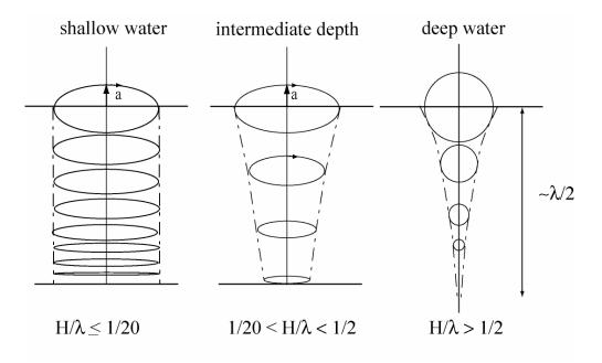
3. Fluid particles move in elliptical orbits below the surface. In deep water, as  $H \to \infty$ , these ellipses become circular.
