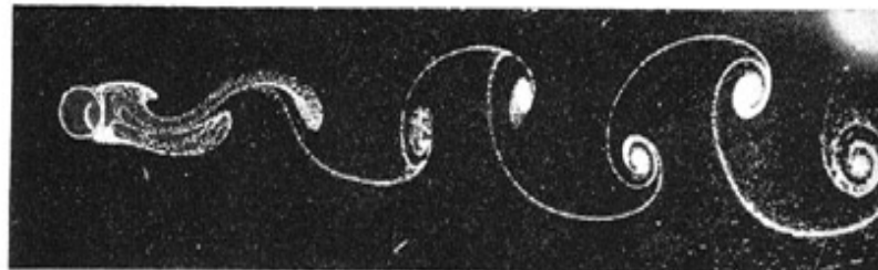
Figure 4.12.6. Streak lines in the wake behind a circular cylinder in a stream of oil. (From Homann 1936a.)
