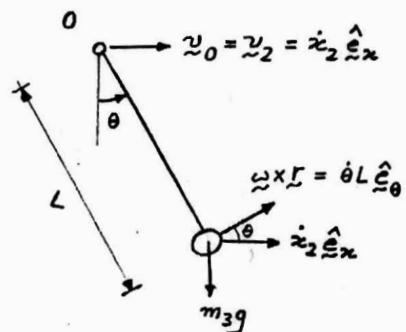
$$\begin{aligned} \underline{h}_0 &= \underline{r} \times \underline{P} = \underline{r} \times m_3 \underline{\omega}_3 = m_3 (L \sin \theta \hat{\underline{e}}_x - L \cos \theta \hat{\underline{e}}_y) \times [(\dot{x}_2 + L\dot{\theta} \cos \theta) \hat{\underline{e}}_x + (L\dot{\theta} \sin \theta) \hat{\underline{e}}_y] \\ &= m_3 (L^2 \dot{\theta} + \dot{x}_2 L \cos \theta) \hat{\underline{e}}_z \end{aligned}$$
