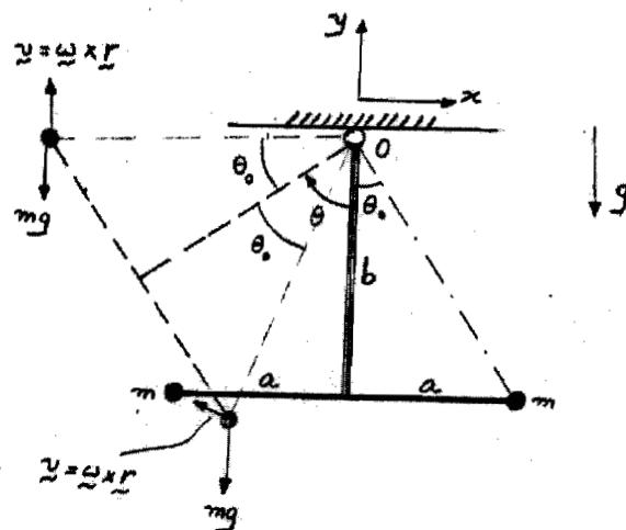
$$\underline{v}_0 = 0 \quad \Rightarrow \quad \underline{\tau}_0^{\text{ext}} = \frac{d\underline{h}_0}{dt}$$
