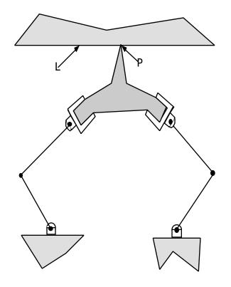
The cooperating robot system shown holds the point P on the line L. What is the mobility of the system?
