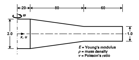
Idealize the structure as an assemblage of 2 two-node elements and calculate the steady-state (pseudostatic) equilibrium equations. (Note that the strains are now  $\partial u/\partial x$  and u/x, where u/x is the hoop strain.)
