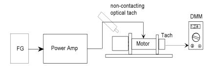
**Procedure:** With the setup as before, remove the torque monitoring lever arm and connect your DMM to the tachometer BNC connector on the motor terminal box. Apply a small dc voltage using the function generator and let the motor spin. The lab instructor will help you to measure the angular velocity with a non-contacting optical
