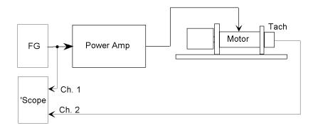
**Procedure:** Set up the function generator to generate a 10% duty cycle, 1 volt unipolar square wave with a 2 second period as follows:
