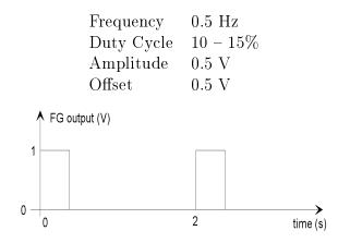
Use the square wave to drive the motor, and record the square wave on Ch. 1 of the oscilloscope, and the angular velocity  $\Omega$  from the tachometer on Ch. 2 of the scope. Adjust the duty cycle to ensure that the motor comes to rest between pulses. Which model of the friction best describes the observed velocity response? Write your answer with reasons below:
