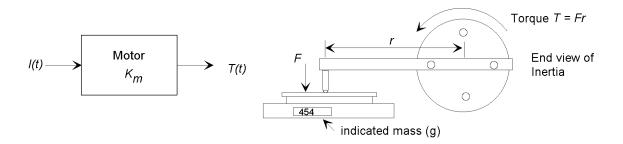
**Procedure** Reconnect the motor to the servo-amp. You are given a digital postage scale and a lever arm that clamps on to the aluminum inertial load. The function generator may be used to generate a given motor current, and the indicated mass shown on the scale may be used to calculate the force applied by the lever arm, and hence the torque.
