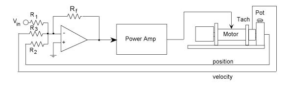
Use the above model to design an implement a position controller that will meet the following step-response performance criteria:
