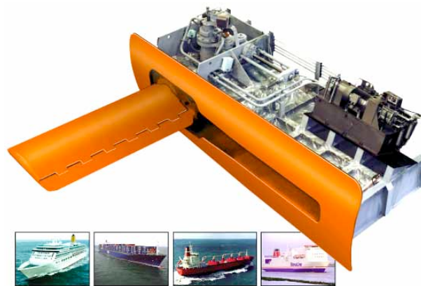
A servo controlled roll fin and hydraulic actuator system
