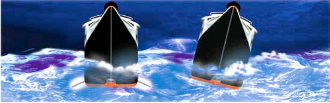
Roll Motion of a ship (right) and lack of roll with stabilizer fins (left)
