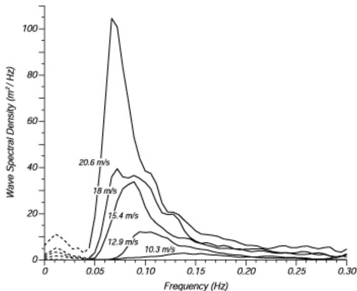
Wave spectra of a fully developed sea for different wind speeds according to Moskowitz (1964).
