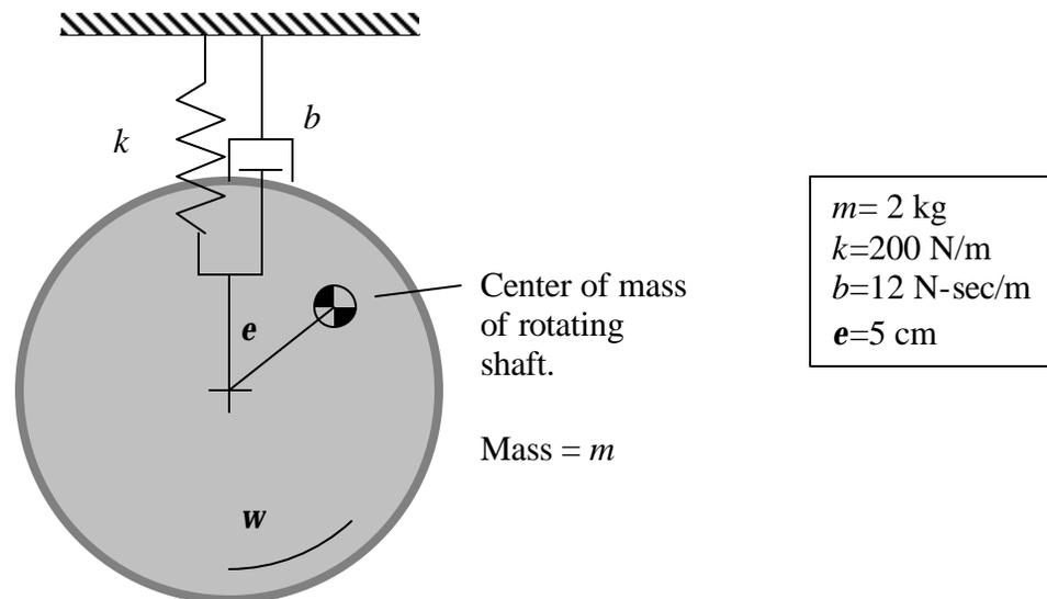
a) Show how we can arrive at a model of the force input to the system that is given by:
