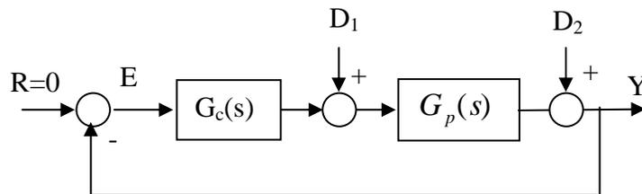
a) Derive the disturbance – error transfer functions  $G_{D_1} = \frac{E(s)}{D_1(s)}$  and  $G_{D_2} = \frac{E(s)}{D_2(s)}$
