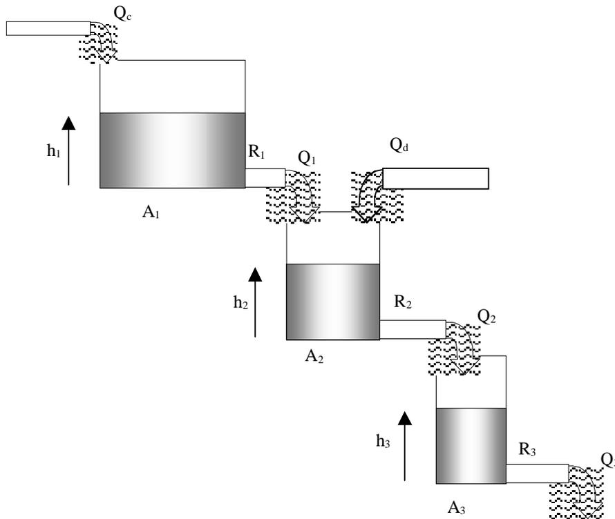
Each tank empties into the next, and there is no back flow (i.e. there is no flow back into the tank from the downstream side).
