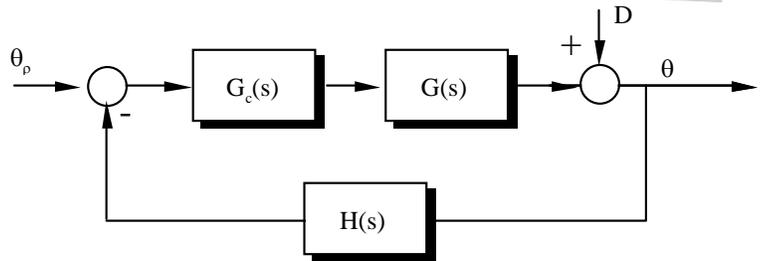
It has been suggested that the angular velocity ( $\dot{\theta}$ ) of the pendulum be measured and fed back in addition to the angle to help in the controlling the system.
