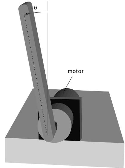
Assume the transfer function relating motor current to pendulum angle is given by:  $G(s) = \frac{10}{(s-1)(s+2)}$
