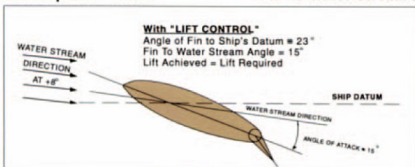
In the above illustrations we show examples of the conditions at a stabiliser fin with and without "Lift Control."
