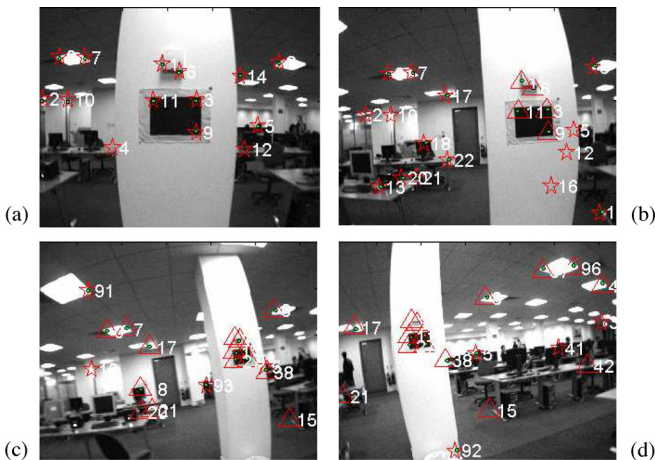
Fig. 15. Parametrization switching seen in image space: points coded in inverse depth (*) and coded in XYZ ( \Delta ). (a) First frame, with all features in inverse depth. (b) Frame #100; nearby features start switching. (c) Frame #470, loop closing; most features in XYZ. (d) Last image of the sequence.
