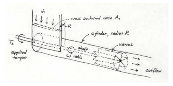
It is clear that the tangential injection causes a swirling flow tends to rotate the vanes in the direction of positive \_\_\_\_\_\_, and the strength of the rotation, or the torque it produces if one holds the vanes static, carries some information about the flow rate.
