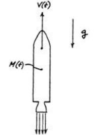
After its second booster has been fired, a space vehicle finds itself outside the earth's atmosphere moving vertically upward against gravity g' at speed  $V_0$ . Its total mass at that point is  $M_0$ . At t = 0, the vehicle's third stage is turned on and the rocket burns propellant at a mass rate of  $\dot{m}_R$  kg/s. Show that if the gravitational acceleration remains essentially constant at the rocket during the firing, the rocket's velocity V(t) after time t will be given by
