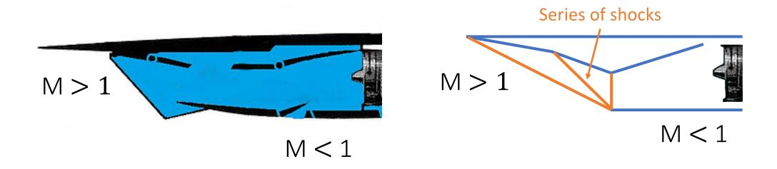
• Objective: minimize total pressure loss for optimal performance
