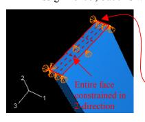
Geometry and loading conditions are exactly the same, but we have to change the boundary conditions on the top left face to eliminate the free rotation around the 2-axis: simply add a constraint in the 1-direction to the
