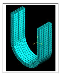
Refine the mesh by changing the local seed on the thickness edges so as to have four elements through the thickness. Rerun the job. Record the CPU time, and obtain new profiles for the axial and transverse shear stresses across the thickness for section B only (9 nodes in the path). Does the shear profile seem more like what you expected? Why?
