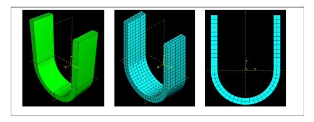
Compare the results of the FE analysis with your pen and paper calculations: by postprocessing the results in the visualization module, try to obtain as many as you can of the quantities evaluated in part (1). As a minimum, you should obtain the numerical value of the following quantities for sections A and C:  $\sigma_{top\ axial}$ ,  $\sigma_{bot\ axial}$ ,  $M_{bend}$ ,  $\sigma_{m\_axial}$ ,  $\tau_{m\_shear}$ .
