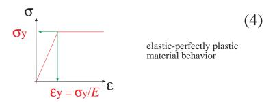
For M>Me the beam is in the elastic-plastic regime: the core of the beam (between y=- c and y=c) is in the elastic regime, while the outer fibers are in the plastic regime ( $\sigma=\sigma_y$ ).
