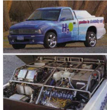
GM (May, 2002) Chevrolet S-10 fuel cell demonstration vehicle powered by onboard reformer
