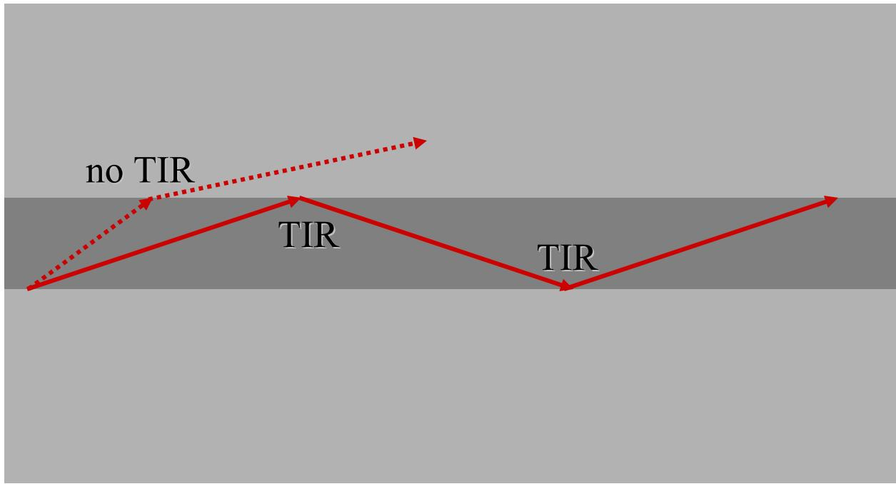
“planar” waveguide: high-index dielectric material
