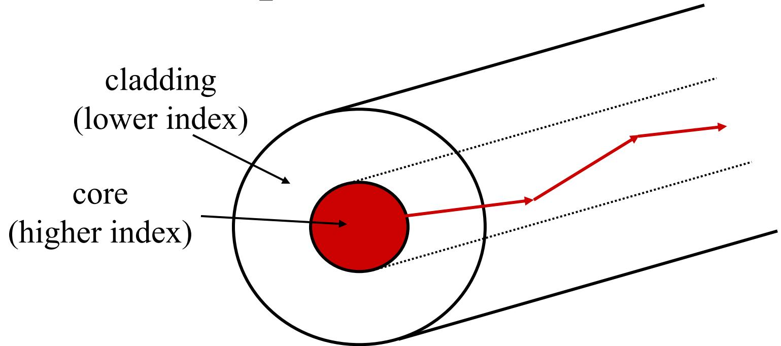
Core diameter =  $8\text{-}10\mu\text{m}$  (commercial grade)
