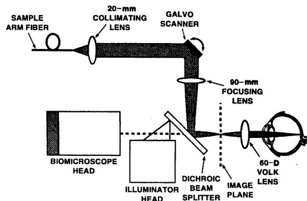
Fig. 2. Schematic of modified slit-lamp biomicroscope. The dichroic mirror combines OCT and the microscope path. Two galvanometric beam-steering devices provide lateral scan (only one axis is shown for simplicity). The 90-mm focusing lens, in combination with the 60-D Volk lens, is designed so as to image the scanning pupil at the patient pupil to eliminate beam shear.
