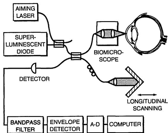
Fig. 1. Schematic of high-speed OCDR system. The system consists of a fiber-optic Michelson interferometer with a superluminescent diode source. High scanning speed is achieved by use of a fast slewing reference mirror. The optical ranging signal is derived by demodulation of the interferometer output at the Doppler frequency. A-D, analog-to-digital converter.
