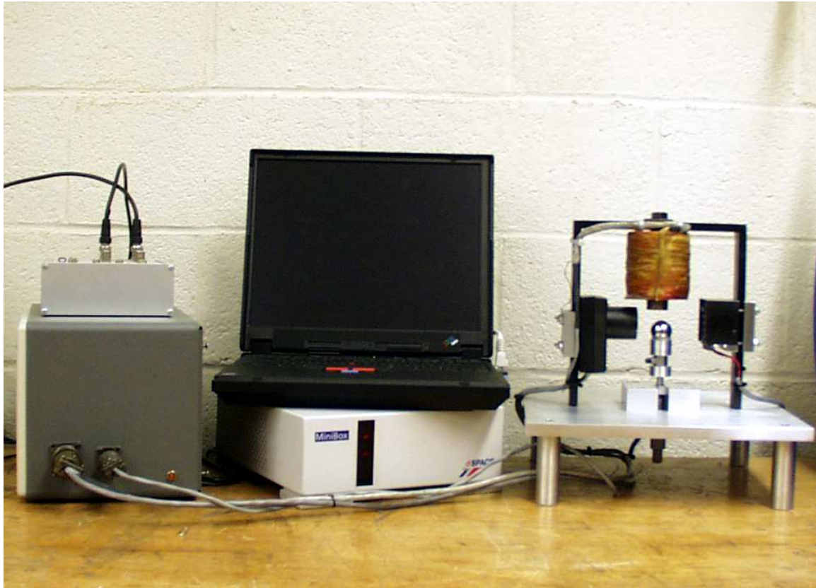
Figure 5-6: Hardware for maglev demo.
