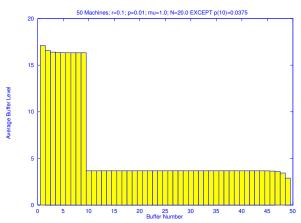
Effect of a bottleneck. Identical machines and buffers, except for  $M_{10}$ .
