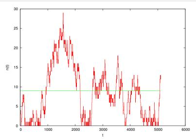
Let  $\rho=\lambda/\mu$ . Under the assumptions of exponential inter-arrival time, exponential service time, and infinite buffer (called M/M/1 queue ), it can be shown that the average number of parts in the system is
