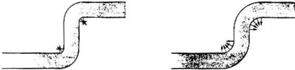
Figure 7.2.24 Identifying hot spots in castings by using outward projecting arrows of length half the casting thickness. Where arrows overlap, hot spots may develop. (Courtesy of Meehanite Metal Corp.)
