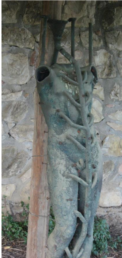
Etruscan casting with runners circa 500 BCE
