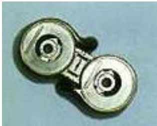
Cores used in Injection Molding
