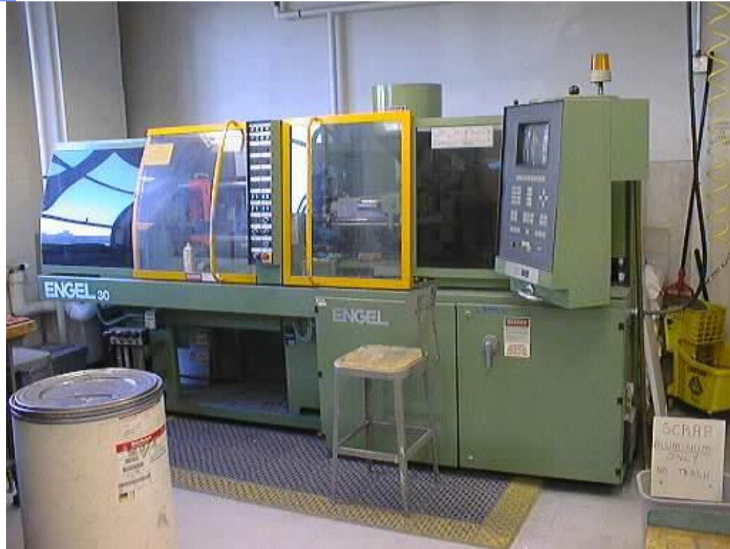
Injection Molding Machine for wheel fabrication
