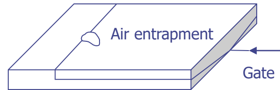
Edge gate: warp free, air entrapment
