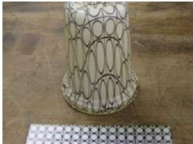
Figure 15-8 Strips of varying width are stretched to obtain different \epsilon_2/\epsilon_1 ratios.
