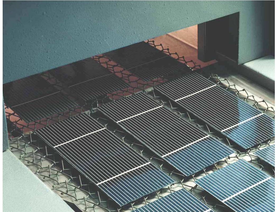
Finished cells emerging from firing of metallization
