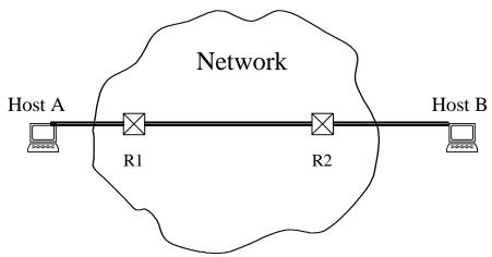
2. *Stop-and-Wait* Assume that hosts A and B are connected to each other via routers R1 and R2. All the links are full-duplex; i.e., the capacity is the same in both directions.
