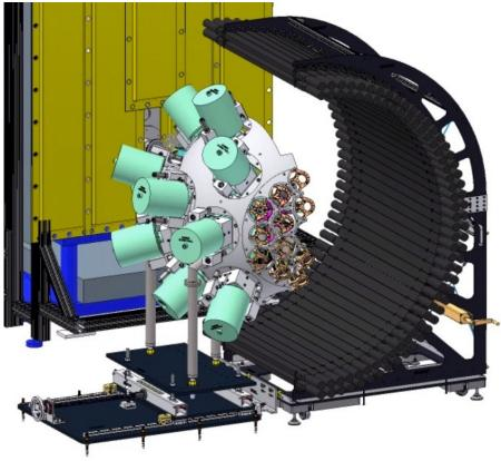
The FRIB Decay Station initiator (FDSi) is being led by ORNL and UTK, and includes (in addition to HPGe), fast timing scintillators, neutron-detection and possibilities for TAS measurements
