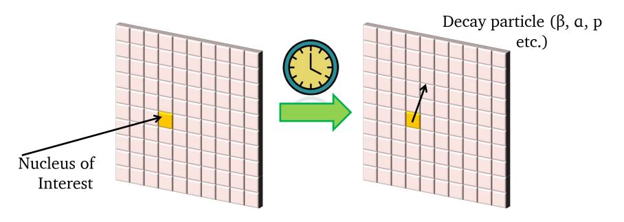
The use of highly-segmented detectors (usually Si) allows temporal and spatial correlations between implanted nuclei, and their subsequent decays → detect the implant and the decay to obtain half-lives and information on levels in the daughter relative to the parent ground state
