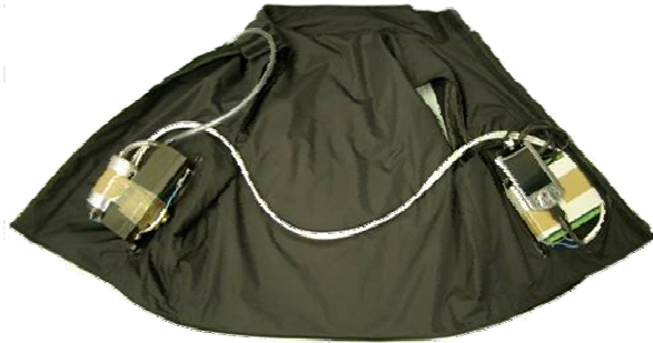
Figure 8. Hug Over a Distance prototype: showing pump, valve, battery, relay controller and wireless PDA. During use, these components are hidden inside the vest.
