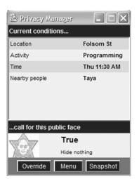
Figure 4. The main screen of the handheld module allows for *in situ* feedback and control. Users could quickly override active preferences and save a snapshot of current contextual variables (*e.g.*, location, time) for subsequent use as a situation parameter. Nested menus offer deeper configuration options.
