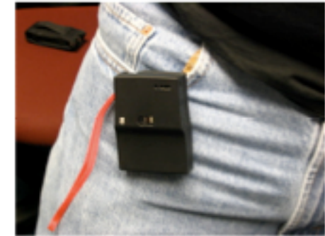
Figure 1 (left) The UbiGreen Transportation Display shows transit behavior as “wallpaper” on a phone’s screen. Here the tree is nearly full of leaves, indicating that the user has completed several green trips for the week. (top) The MSP sensor worn near the waist and the phone’s GSM cell tower data are used to semi-automatically infer transportation mode.
